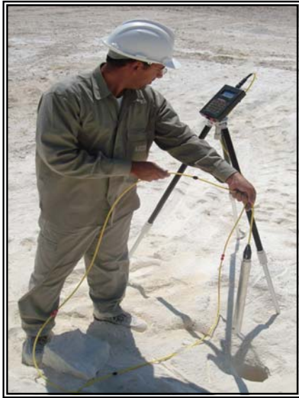
Fig. (7) Cabled Boretrak instrument.
