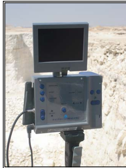
Fig. (12) High speed digital video camera.
